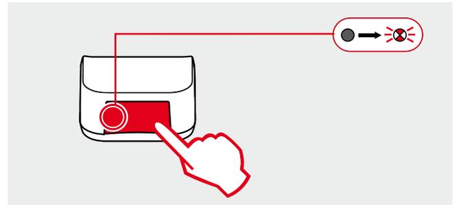
2. Press the NETWORK key again for at least 10 seconds. The NETWORK LED will flash quickly twice and then will turn off. The interface is no longer connected to the ZigBee network.
