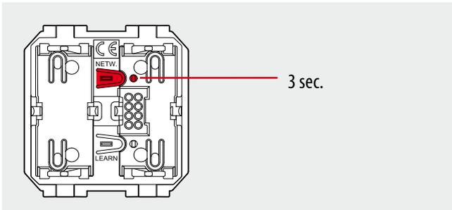
2. The NETWORK LED (yellow) will come on steady, and after a few instants will start flashing quickly.
