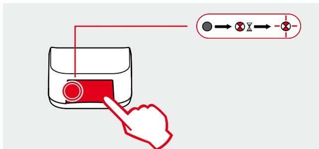
4. To complete the procedure press the NETWORK KEY of the Coordinator device; the corresponding NETWORK LED will flash three times while the interface NETWORK LED will turn off.
