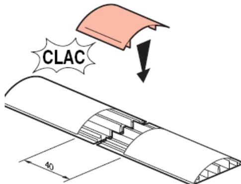
For mounting with floor ducts 92x20mm
