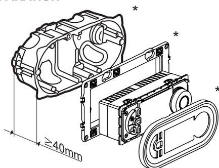
\* not delivered with the mechanism
