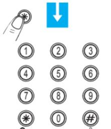
Confirm the selection using the user code, a transponder key or a numeric code
