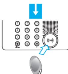
In case of a technical alarm (its symbol appears), you can find out which device has produced the alarm and reset it as well.
